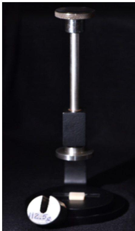
Figure 29. Metlab Sample Leveling Press Device
