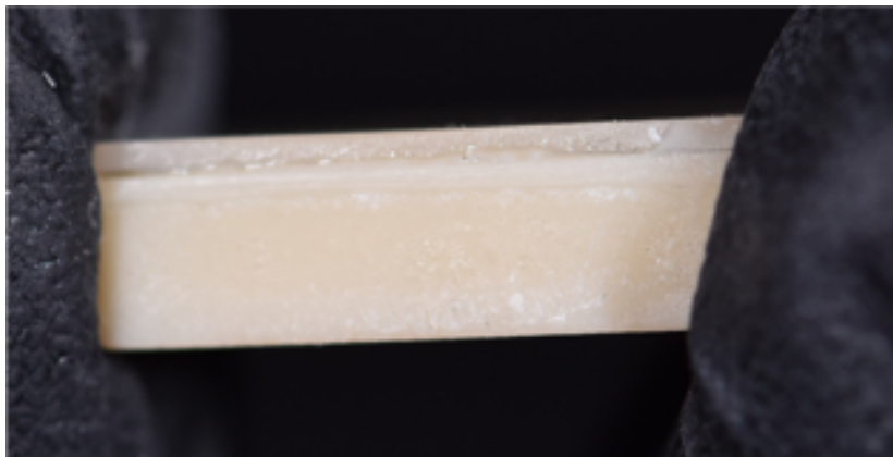
Figure 33. Specimen After Removal of Excess Cement
